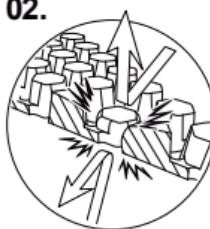
02 » Deformation of the structure results in impact absorption and internal dispersion
